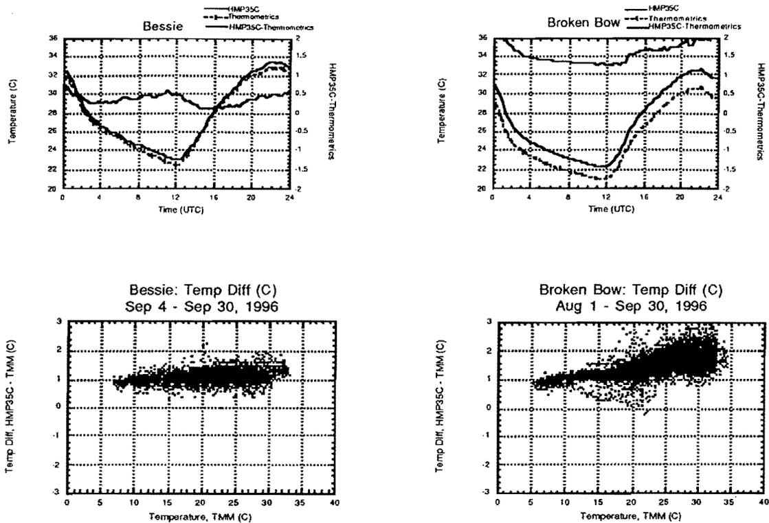
Figure 2: Temperature measured using the HMP35C and Thermometrics (TMM) at 1.5 m.
