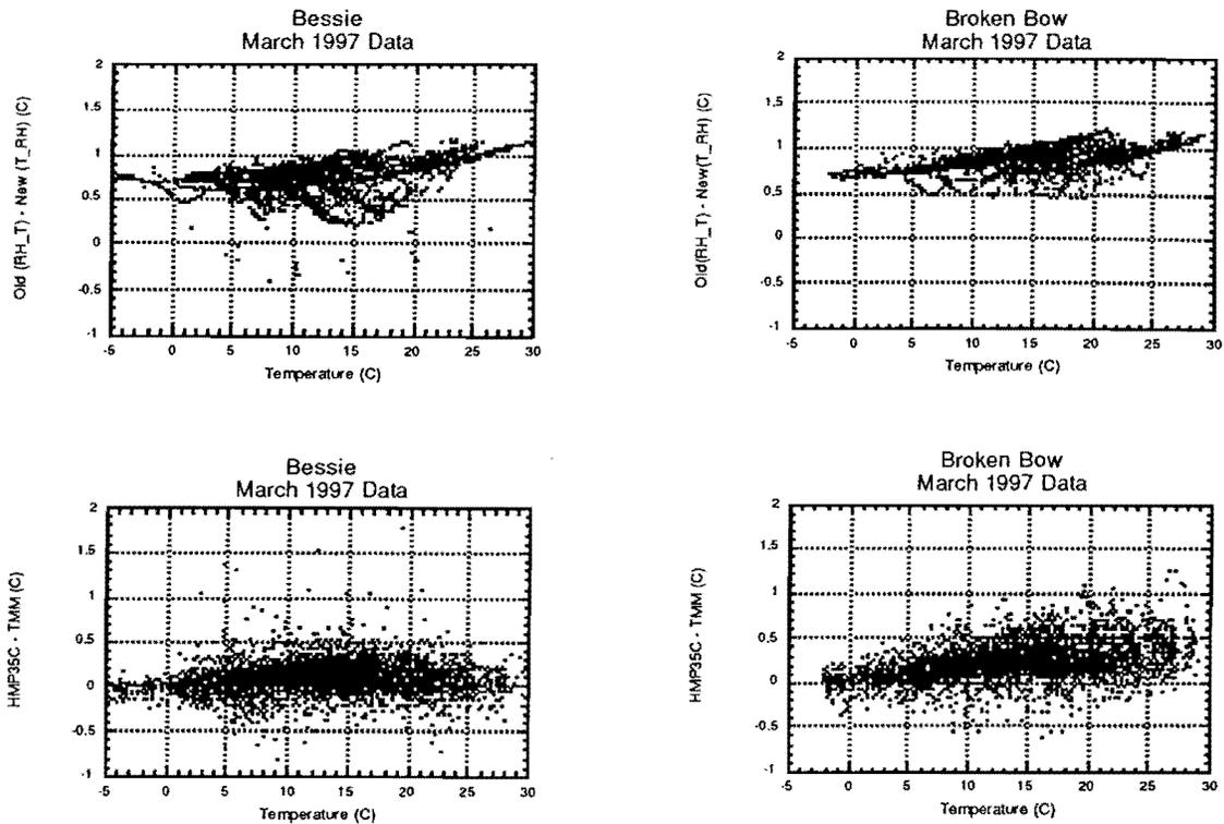
Figure 3: a) (Top): The temperature difference between the old (RH\_T) and new (T\_RH) methods of measuring the HMP35C air temperature.
